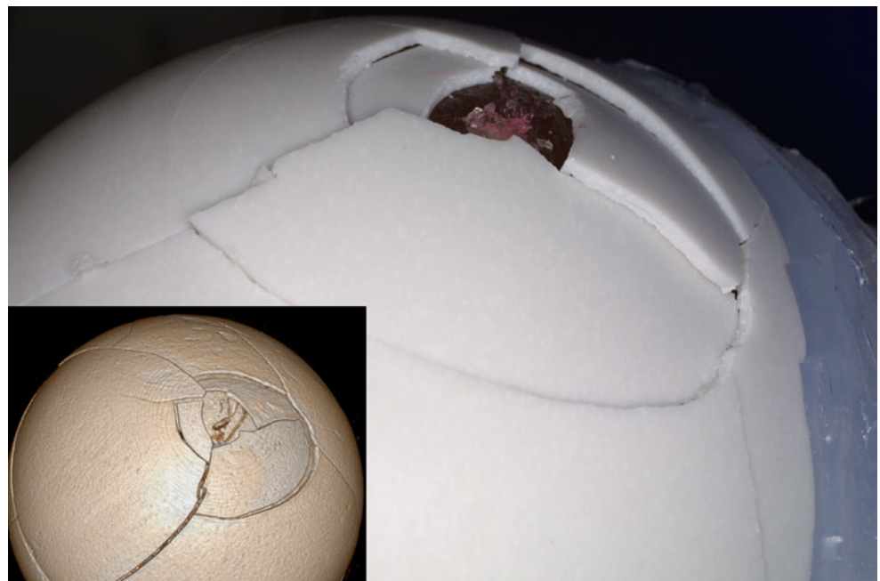
Fig. 2 Exit hole of the polypropylene model after removal of the silicone coat. The volume rendering of CT image data realistically displays the fractures of the bone simulant
